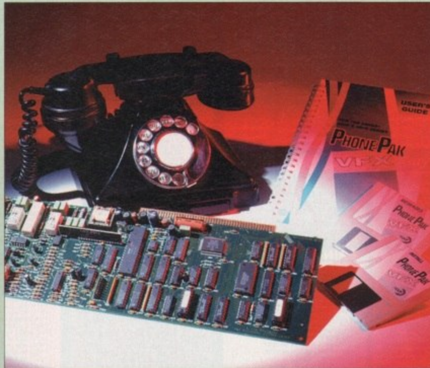
Phone-Pak – a fax, answering machine and voice mail system all in one package
